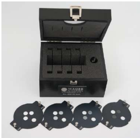
Figure 5: Optical Validation Kit consisting of traceable standard Neutral Density Optical Filters, which are inserted into the AE33 optical path to determine the reproducibility of the relationship between LED optical source intensity and detector response.
