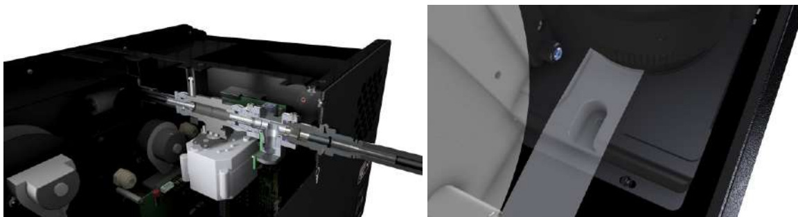
Figure 12. Two RH sensors were installed in AE36s. The left position of the RH sensor is in the inlet line, and the right RH sensor is in the filter tape compartment.
