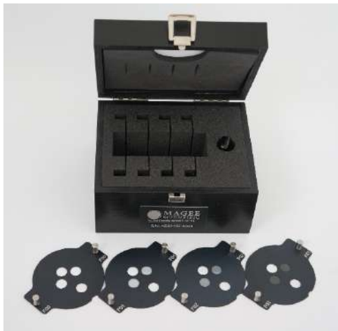
Figure 16. The Optical Validation Kit consists of traceable standard Neutral Density Optical Filters inserted into the AE36s optical path to determine the reproducibility of the relationship between LED optical source intensity and detector response.
