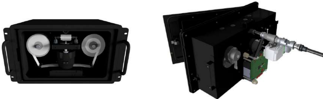
Figure 10 Filter compartment of AE36s from the front and backside. Hermetic seals prevent dust and moisture ingress in the vicinity of filter tape.
