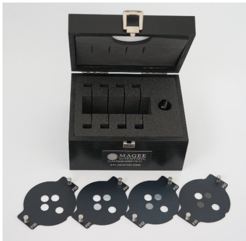
Figure 11. The optical Validation Kit consists of traceable standard Neutral Density Optical Filters inserted into the AE36 optical path to determine the reproducibility of the relationship between LED optical source intensity and detector response.
