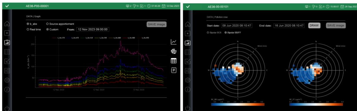
Figure 8. Graphical data presentation on AE36- timeseries of absorption coefficient at 7 wavelengths left, and Pollution rose right.
