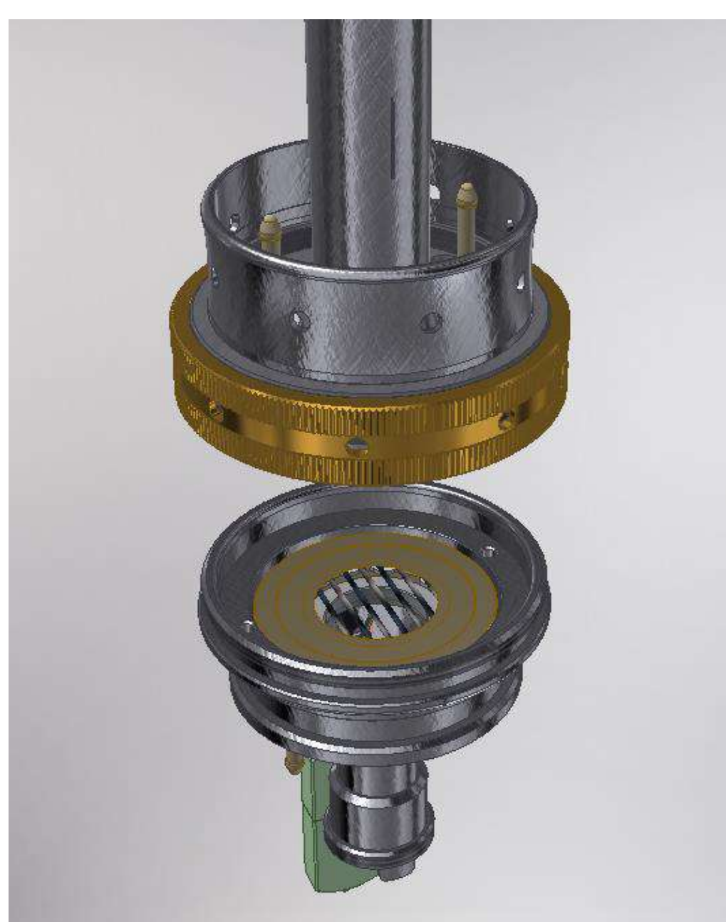
(3) Combustion chamber in TCA-08.
